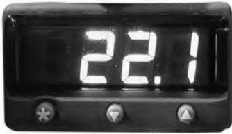
Temperature monitor/controller display and buttons.
