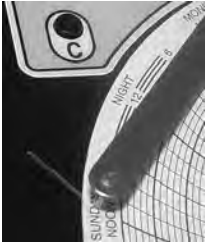
Chart recorder stylus and time line groove
