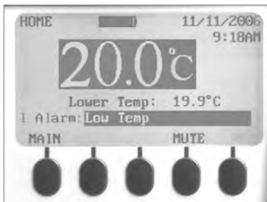
Home screen with one active alarm (Low Temp), highlighted.
