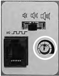
Alarm delay control (circled).
