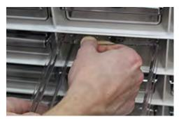
Tab on outer edge engaged with slot
