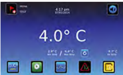
Figure 3: Home screen with no alarms.
