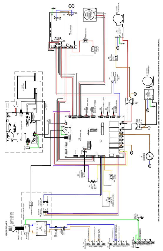
8.2 Electrical Schematic (Units with serial number 2149917 and beyond)
