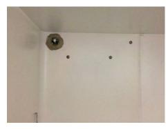
Threaded screw holes and distribution port for back-up refrigeration system installation
