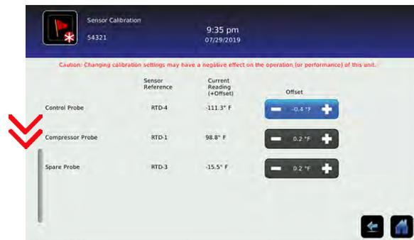
Sensor calibration values are programmed at the factory. Calibration values can be viewed and changed through the i.C<sup>3</sup> monitoring and control system.
