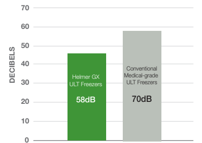
Every increase of 10dB on the scale is equivalent to a 10-fold increase in sound intensity.
