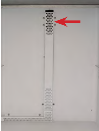
Chamber temperature sensor (located behind cover).
