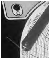
Chart recorder stylus and time line groove
