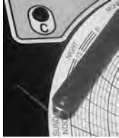
Chart recorder stylus and time line groove
