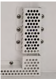
Chamber temperature sensor (located behind cover).
