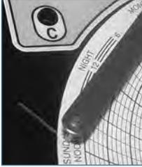
1. Press and hold C button. When stylus begins to move left, release button. The LED flashes.
