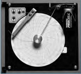
The chart recorder has a back-up battery system enabling a period of continuous operation if power is lost. Battery life varies by manufacturer as well as voltage level remaining. If full battery power is available, back-up power for the temperature chart recorder is available for up to 14 hours.
