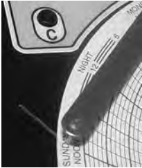
Chart recorder stylus and time line groove
