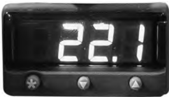
Temperature monitor/controller display and buttons.
