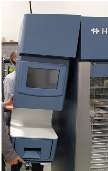
*Compartmental Access Refrigerator and Access Console assembly*
