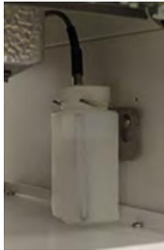
*Primary probe (with probe bottle and bottle holder)*
