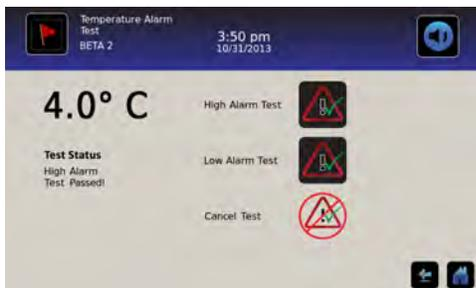
Temperature Alarm Test screen
