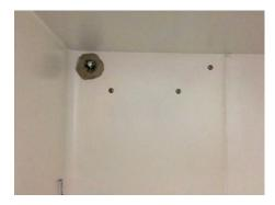
Threaded screw holes and distribution port for back-up refrigeration system installation
