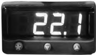
Temperature controller display.
