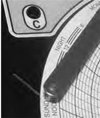
*Chart recorder stylus and time line groove*
