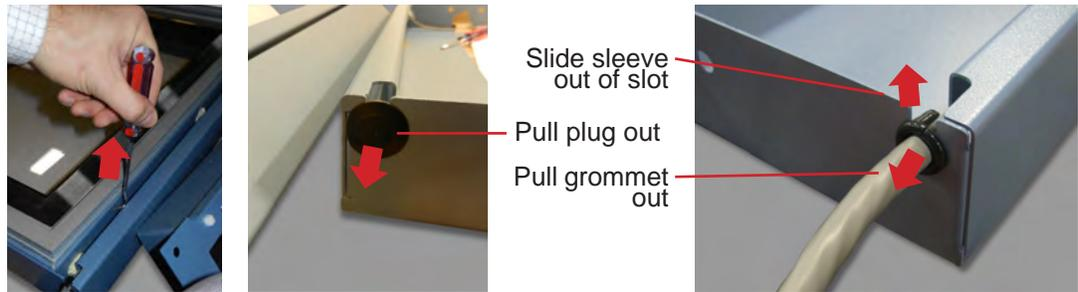
Left: Remove the inner door with a J-hook tool.
