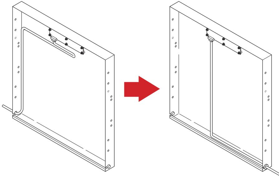
Left: Original cable routing (wired for right-hinged door).
