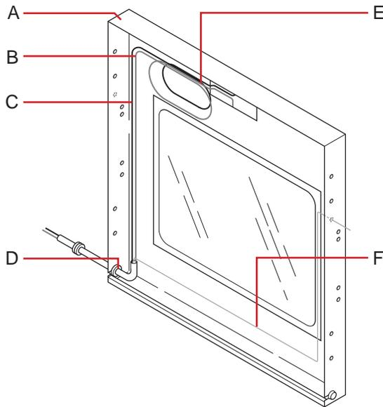
Outer door frame (right-hinged door shown), power and communication cables, and optional Access Control cable.
