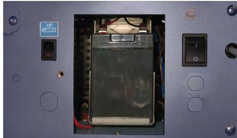
Monitoring system backup battery (access panel removed).
