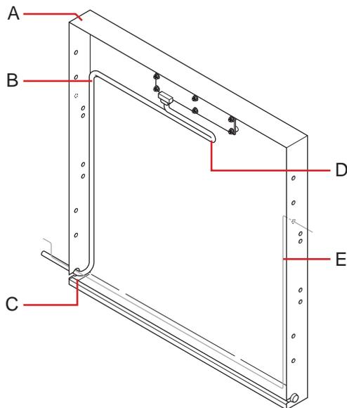
Outer door frame (right-hinged solid door version shown), data cable, and optional Access Control cable.
