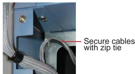
Power and communication cable(s) secured at hinge-side of the cabinet after hinge reversal.
