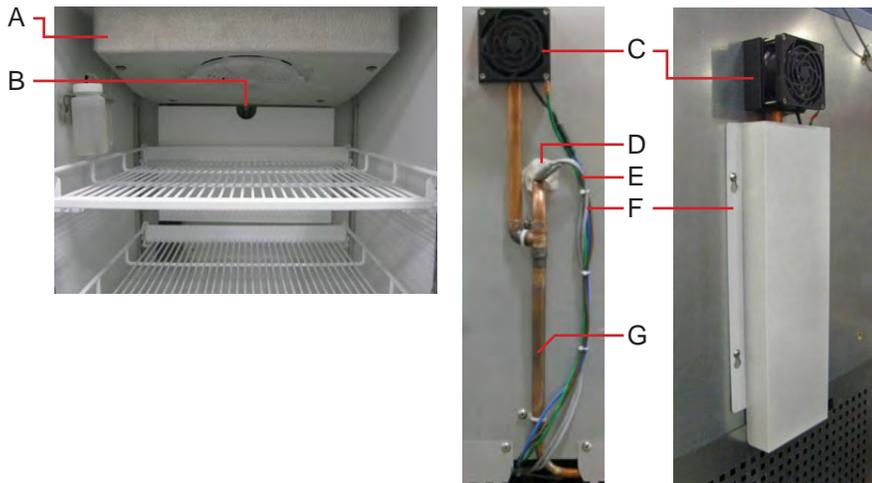
Left: Unit cooler (A) inside the chamber, with drain port (B).
