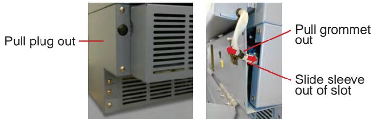
Left: Remove the plug from the access panel.
