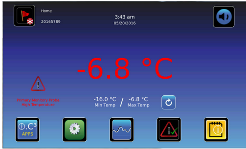
Home screen with active alarm
