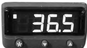
Temperature controller display.
