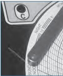
Chart recorder stylus and time line groove
