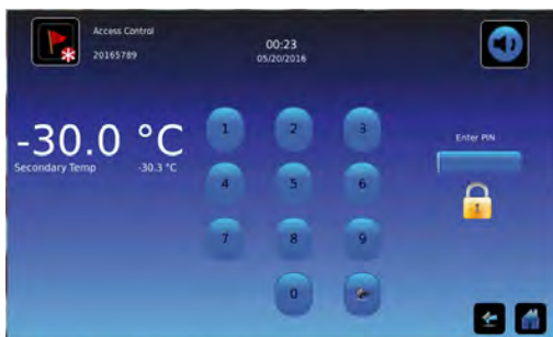
Access Control Keypad
