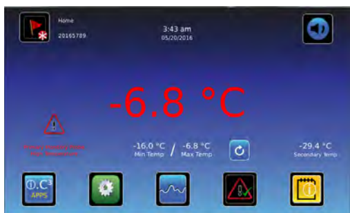
Home screen with active alarm
