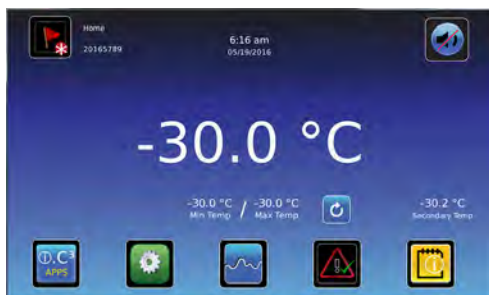
Home screen - alarm muted
