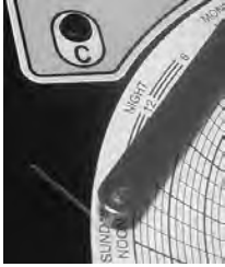
Chart recorder stylus and time line groove
