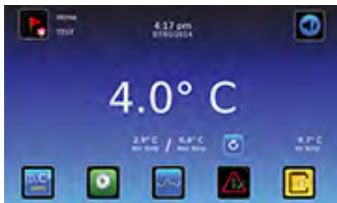
Figure 13: Home screen with no alarms.
