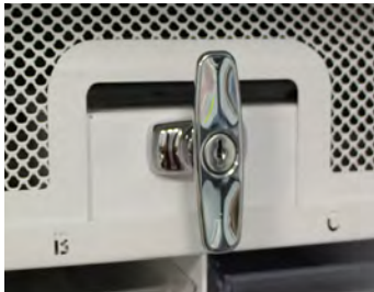
Figure 20 (left): Bypass Release handle and lock (shown in unlocked position).
