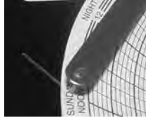
Figure 3: Chart recorder stylus and time line groove.
