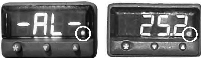
Temperature monitor/controller in alarm condition (red lamp circled).
