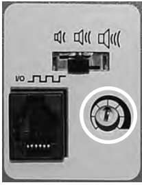
Alarm delay control (circled).
