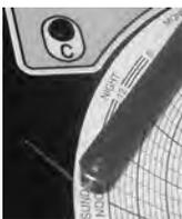
*Chart recorder stylus and time line groove*
