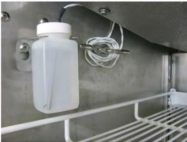
Left: Probe bottle with temperature probe
