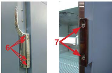
6. Remove four screws securing door handle assembly to door and set assembly aside.
