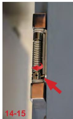
11. Orient bend in coil toward front of freezer and slide internal hex cap with washer onto upper hex bolt in lower hinge plate.
