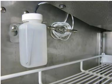
Left: Probe bottle with temperature probe
