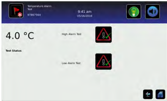
Temperature Alarm Test screen
