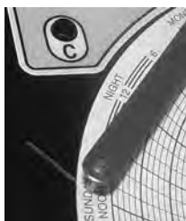
Chart recorder stylus and time line groove
