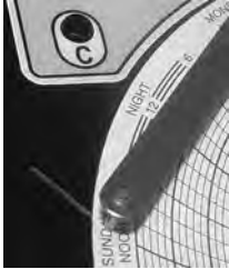
Chart recorder stylus and time line groove
