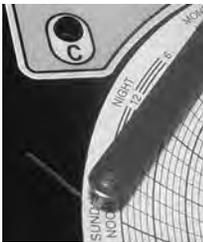
Chart recorder stylus and time line groove
