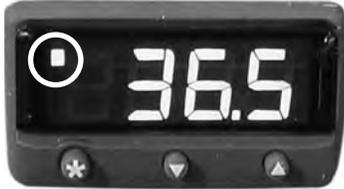
*Temperature controller with chamber heater light (circled).*
