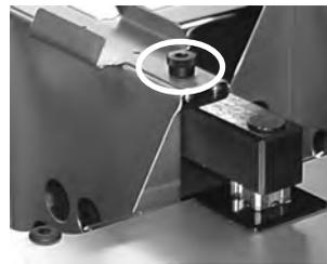
Basket installed on lift-out arm. Finger knob circled.
