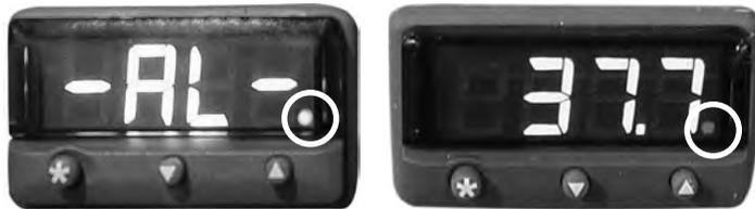
*Temperature controller with a high temperature alarm. Alarm light is circled.*
