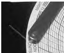
Chart recorder stylus and time line groove
