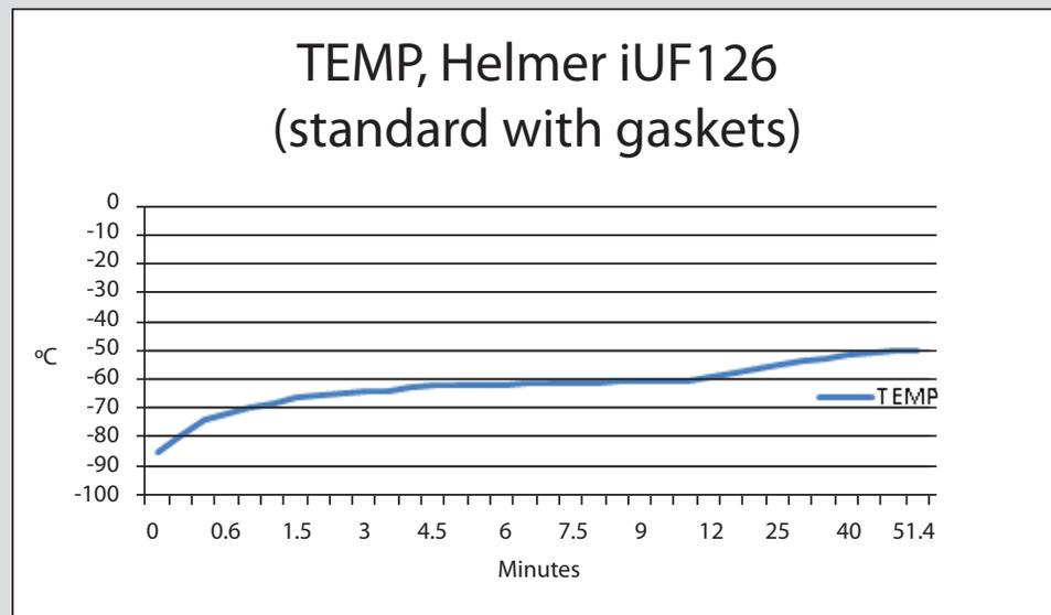
The time for the average cabinet temperature to reach -50°C with the outer door and top inner door open was 51.4 minutes.
