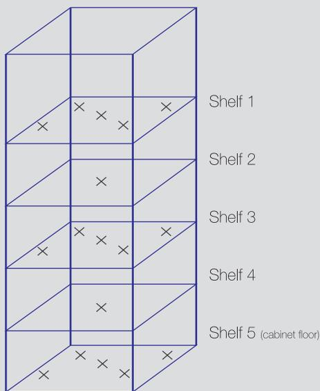
The cabinet temperature average used for these tests is the average of the individual shelf average temperatures. Time is in minutes, with 0 indicating the time of the last measurement before the door opening. Temperature is in degrees Celsius. The set temperature of the ultra-low freezers was -86°C and ambient temperature was 24°C, +/- 1°C. The units were tested with both compressors running throughout the warmup period.
