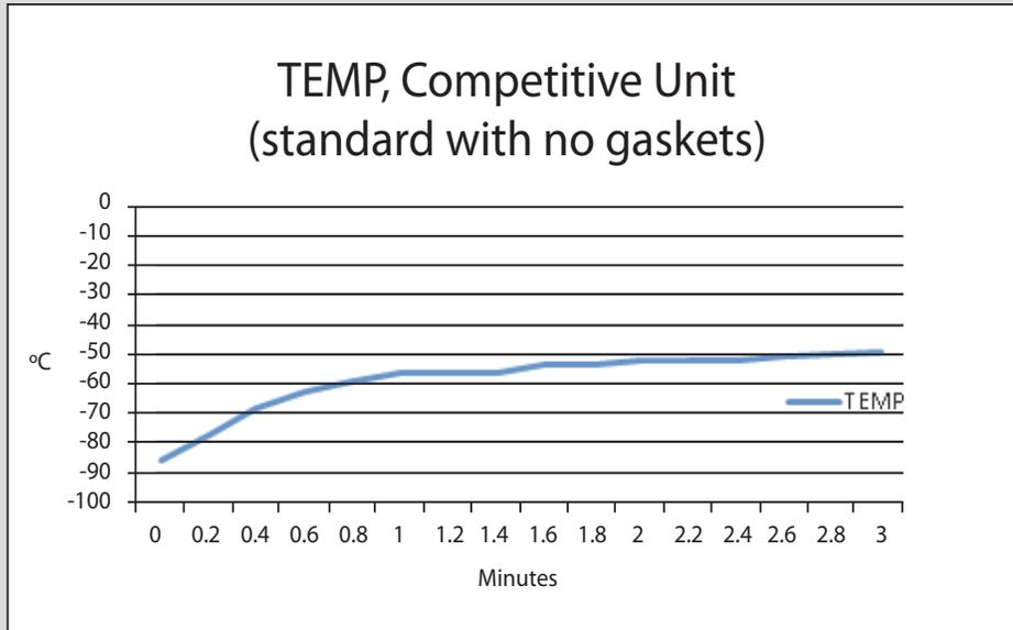
The time for the average cabinet temperature to reach -50°C with the outer door and top inner door open was 3 minutes.
