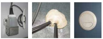
Left: Probe bottle with temperature and chart recorder probes. Middle: Access port as seen from the top of the refrigerator. Right: Access port on side of refrigerator. The number and location of ports varies by model.
