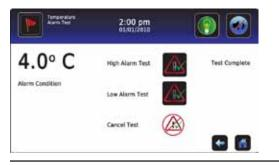
The automatic test can be aborted at any time by touching the **Cancel Test** button.
