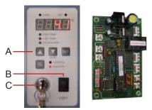
Left: Display with touchpad. Right: Rear view of display, showing monitor/control board.
