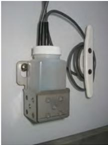
*Probe bottle with temperature probes*
