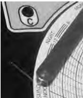
*Chart recorder stylus and time line groove*
