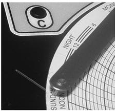
Chart recorder stylus and time line groove.
