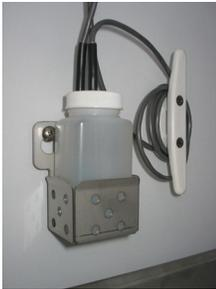
*Probe bottle with temperature probes*
