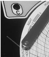
*Chart recorder stylus and time line groove*
