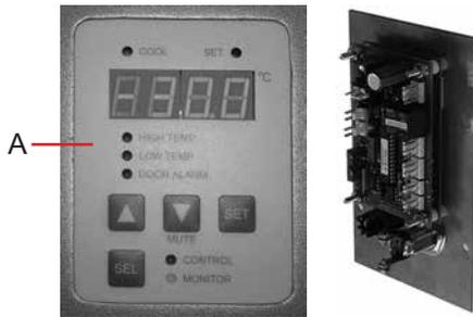
Left: Laboratory display with touchpad. Right: Rear view of display showing monitor/control board.
