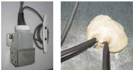
Left: Probe bottle with temperature and chart recorder probes. Right: Access port on the top of the freezer. The number and location of ports varies by model.
