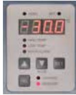
Horizon Series temperature monitor and controller.
