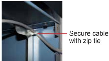
*Data cable secured at the hinge-side of the cabinet after hinge reversal.*
