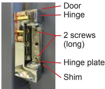
Attach hinge to door (lower hinge shown).
