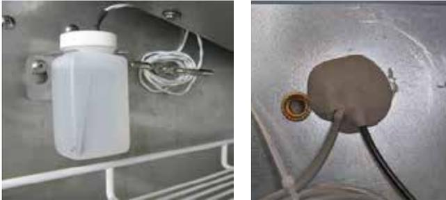
*Left: Probe bottle with temperature probe. Right: Access port on rear of refrigerator.*
