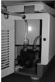
Access door open with pump visible.
