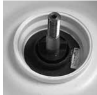
Rotor shaft / motor hub removed.
