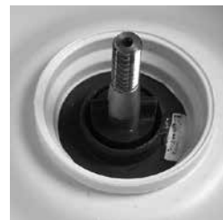
Seal correctly adjusted.
