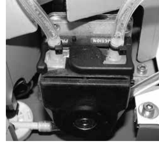
Holder locked in position around pump. Right side of tubing connected to flow meter fitting.
