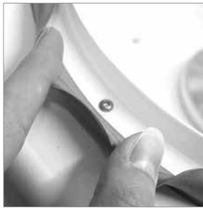
Gasket folded back and section of lower drainage ring removed.
