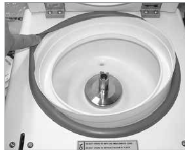
Entire lower drainage ring loosened.
