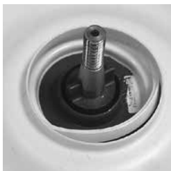
Seal partially pinched under the bowl.
