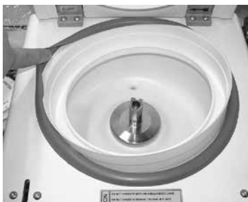
Lower drainage ring placed in the bowl.
