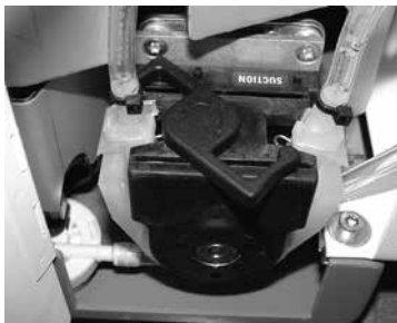
Pump with loosened tubing holder.
