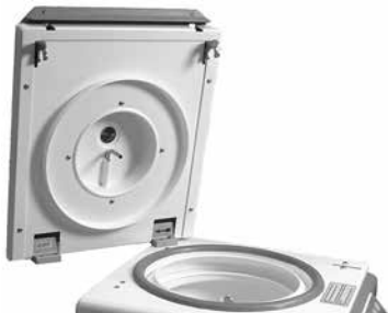
Lid loosened and swung away from the cell washer.
