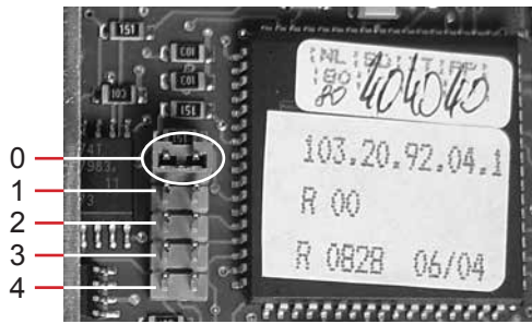
Jumpers configured for normal operating mode.
