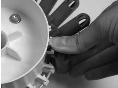
Bottom of rotor with tube holder being removed.
