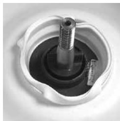
Seal pulled toward shaft, with edges partially pulled around edge of the center hole.
