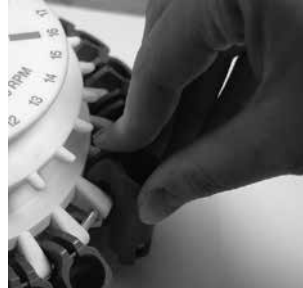
Tube holder being installed.
