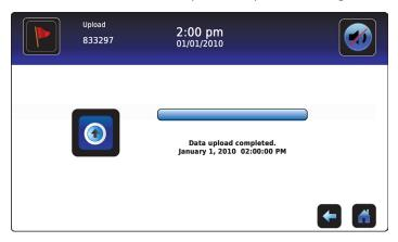
4. After the "Data Upload Completed" screen is displayed, the screen refreshes to display the "Wait" screen. The system automatically powers down and restarts.
