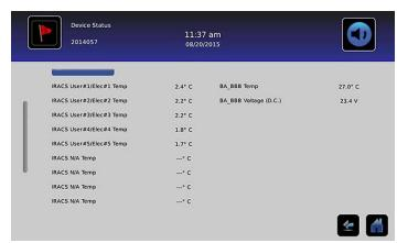
Device Status is divided into two sections. The upper section records the current status of the refrigerator components while the lower section allows viewing of the status of the compartmental access system. The **Refresh** button, when selected, will update the temperature readings of the IRACS boards and BA\_BBB as well as the voltage reading of the BA\_BBB.
