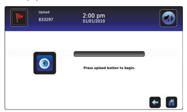
**Note:** If the Upload icon is touched before a memory device is inserted, the message "Insert USB Flash Drive" is displayed until a memory device is inserted.
