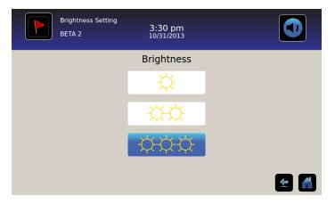
The backlight on the i.C<sup>3</sup> monitor has three (3) settings.
