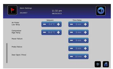
The setpoint is the temperature at which the temperature alarm is activated.
