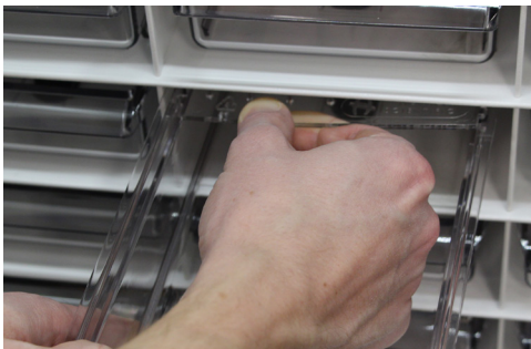
Tab on outer edge engaged with slot
