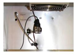
The glycol sample bottle temperature probe must be fully inserted into the glycol sample bottle in order to monitor the temperature of the substance in the bottle.
