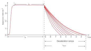
B-ramps enable the buckets to return to a vertical position gently and without vibration before coming to a stop.
