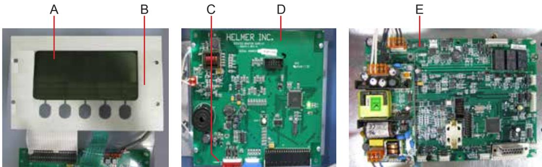
Left: Display assembly including LCD display and touchpad. Middle: Display board. Right: Control board.
