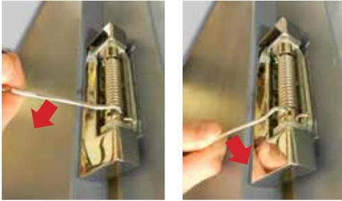
*Rotate the spring using a J-hook tool then insert pin (left-hinged door shown).*
