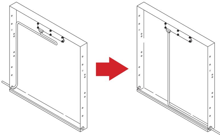
*Left: Original cable routing (right-hinged door). Right: New cable routing (left-hinged door).*
