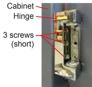
Attach hinge to cabinet (lower hinge shown).
