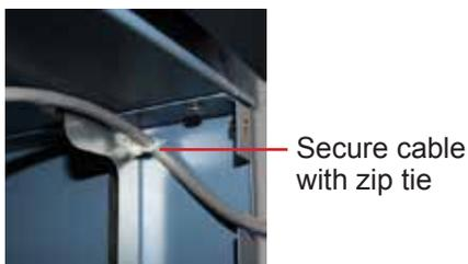
Data cable secured at the hinge-side of the cabinet after hinge reversal.
