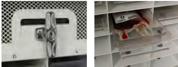
Figure 20 (left): Bypass Release handle and lock (shown in unlocked position).
