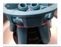
**NOTE** Do not discard the rubber band, transport bolts, sleeves, and transport fittings. If the centrifuge must be returned for service, the transport hardware must be reinstalled.
